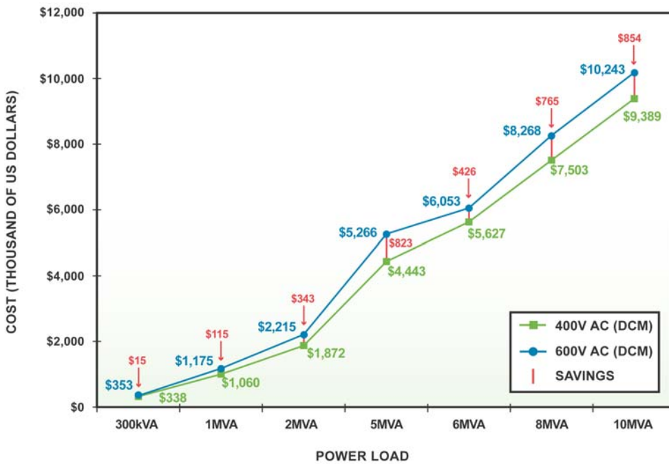
Chart 7: First-year TCO (400V AC vs. 600V AC, both in double conversion mode)
