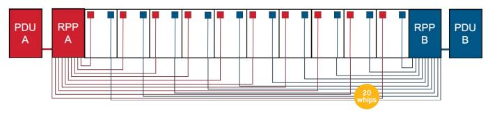
30A Z-PDS DEPLOYMENT (Two PDUs, zero RPPs, 10 + 2 extra racks, and 12 whips)
