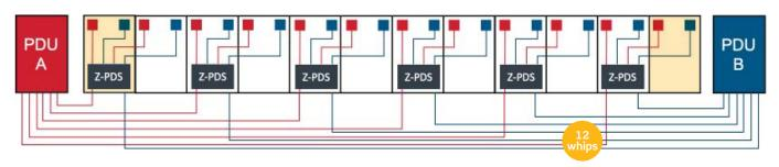
20A Z-PDS DEPLOYMENT (Two PDUs, zero RPPs, 10 + 2 extra racks, and 8 whips)
